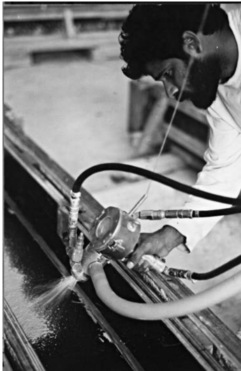
Figure 33.8 Dual-spray concentric nozzle system for glass-frc. The large pipe at the bottom right of the spray gun supplies matrix; the small straight metal pipe at the top left is the roving intake. The black pipes supply compressed air to both power the roving chopper and propel the chopped fibre and matrix. (Supplied by Iain D Peter, Powersprays Ltd., http://www.powersprays.com )
