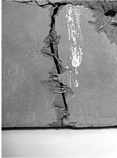
Figure 32.9 Fibres bridging a crack in steel-frc.
