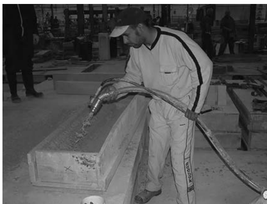
Figure 33.7 Spraying of premix glass-frc. (Supplied by Iain D Peter, Powersprays Ltd., http://www.power-sprays.com/ )
