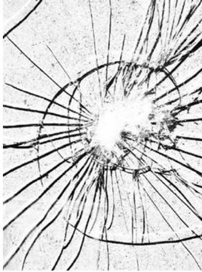
Figure 38.4 Breakage pattern of laminated annealed glass.
