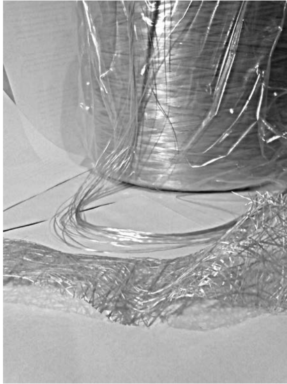
Figure 28.2 Glass fibres for FRC. Foreground – chopped strand mat. Background – continuous roving for chopping.
