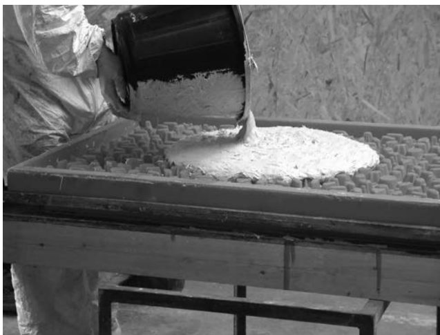
Figure 33.6 Manufacture of a cast premix glass-frc cladding panel. (Supplied by Iain D Peter, Powersprays Ltd., http://www.power-sprays.com/ )
