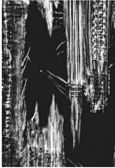
Figure 43.8 Tensile failure in spruce ( Picea abies ) showing mainly transverse cross-wall failure of the earlywood (left) and longitudinal intra-wall shear failure of the latewood cells (right) ( \times 110 , polarised light). (Copyright Building Research Establishment.)
